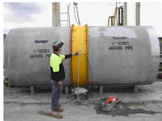
Figure 3 - External Hydrostatic Testing
