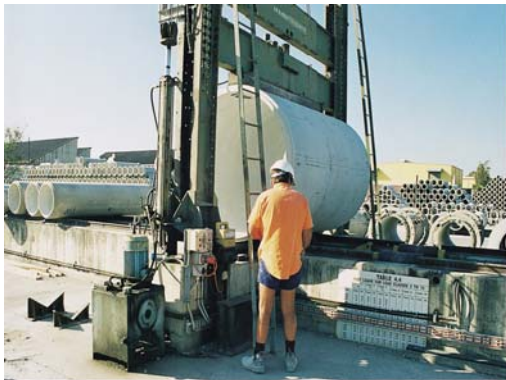
Figure 2 - Pipe External Load Testing
